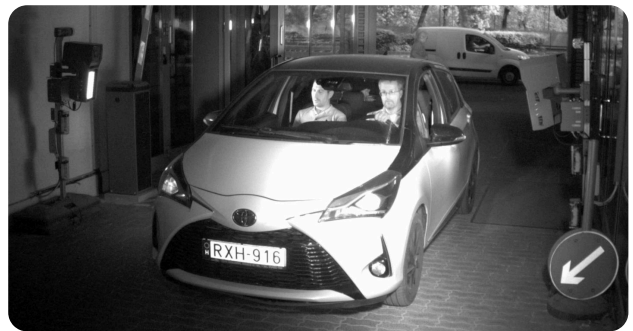
FIGURE 3 Front, IR sensor. Driver and front passenger through the windscreen.
