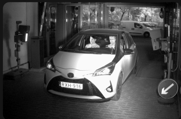
760 NM NEAR-INFRARED The same vehicle, occupants visible through the windscreen.
