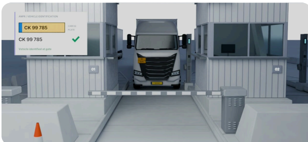
FIGURE 1 The plate is read as the truck pulls up and posted to the check-in system.
